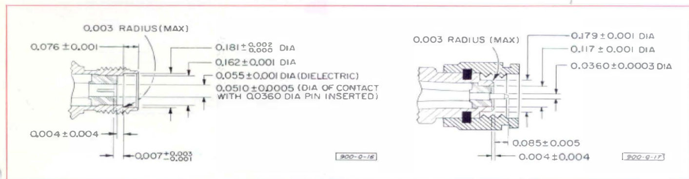
Figure 4. Critical mating dimensions for Types 874-QMMJ and -QMMP Adaptors.
